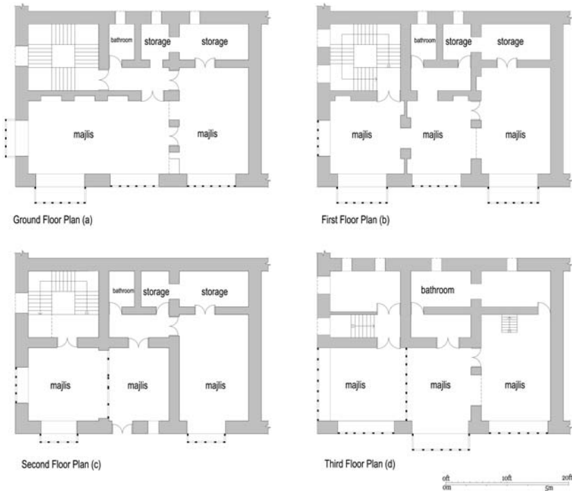
Figure 7. Plans of the bottom four floors of a five-story house in Jidda, Saudi Arabia. Drafted by Anwar Ibrahim, adapted from Bonenfant, “La maison dans la péninsule arabique,” 775–776.
